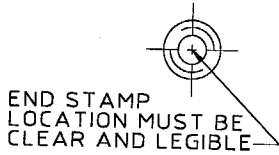
FIGURE 2 EXPOSED END OF THE ANCHOR IS STAMPED TO IDENTIFY ANCHOR LENGTH. STAMPINGS SHOULD BE PRESERVED DURING INSTALLATION FOR ANY SUBSEQUENT EMBEDMENT VERIFICATION. (SEE TABLE 2)
